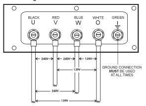
Figure 22. Output Terminal Lugs 3Ø-240/139V Connections
